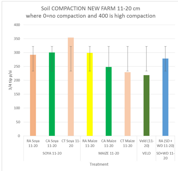
Figure 15 Soil compaction measured with a penetrometer at New Farm trial at 11-20cm
