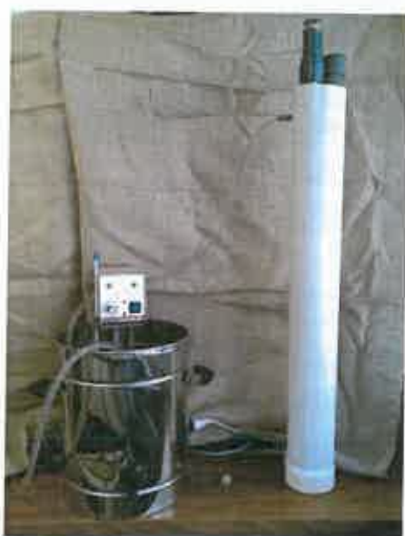
Plate 5.4-1: Thermistor calibration set-up.
