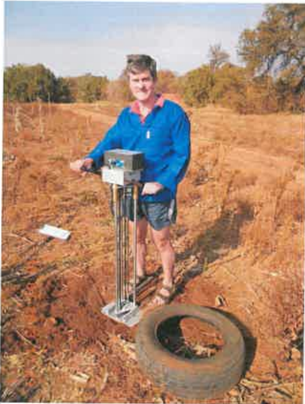
Plate 5.5-2: Measuring soil penetration resistance with a penetrometer, as indicator of soil compaction. The tyre was used to help wet the soil in preparation for sampling.
